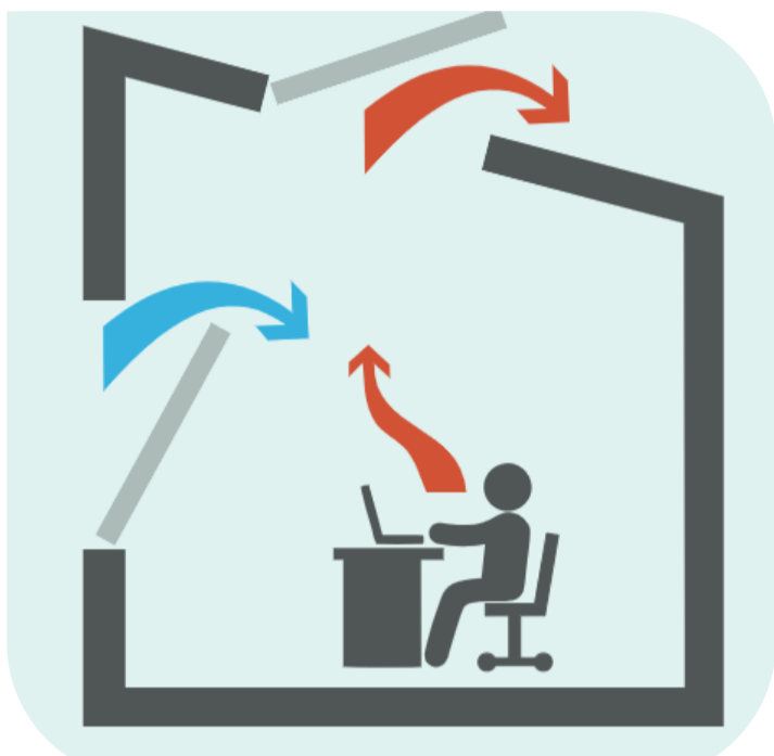
Diagram of the stack effect (chimney effect) in a room [Wikipedia]
