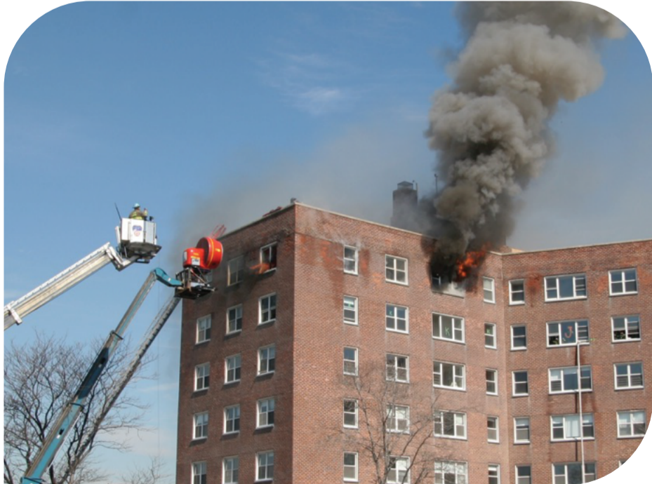
A fan, simulating wind, changes airflow and smoke conditions during experiments in a seven-story high-rise abandoned apartment building on New York City's Governors Island [Wikipedia]
